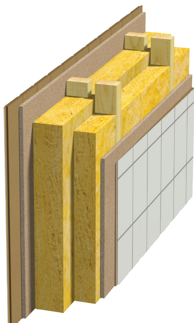
Fig. 4 Internal wall Double wood studs on double wood sill. Double boards.
