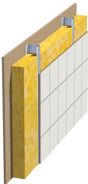
Fig. 5 Internal wall All through steel studs. Single board.
